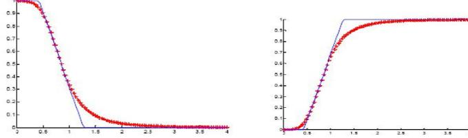
Figure 2: shows the approximation of hill function by piecewise multi-affine function, Better approximations can be obtained by using more breakpoints.
