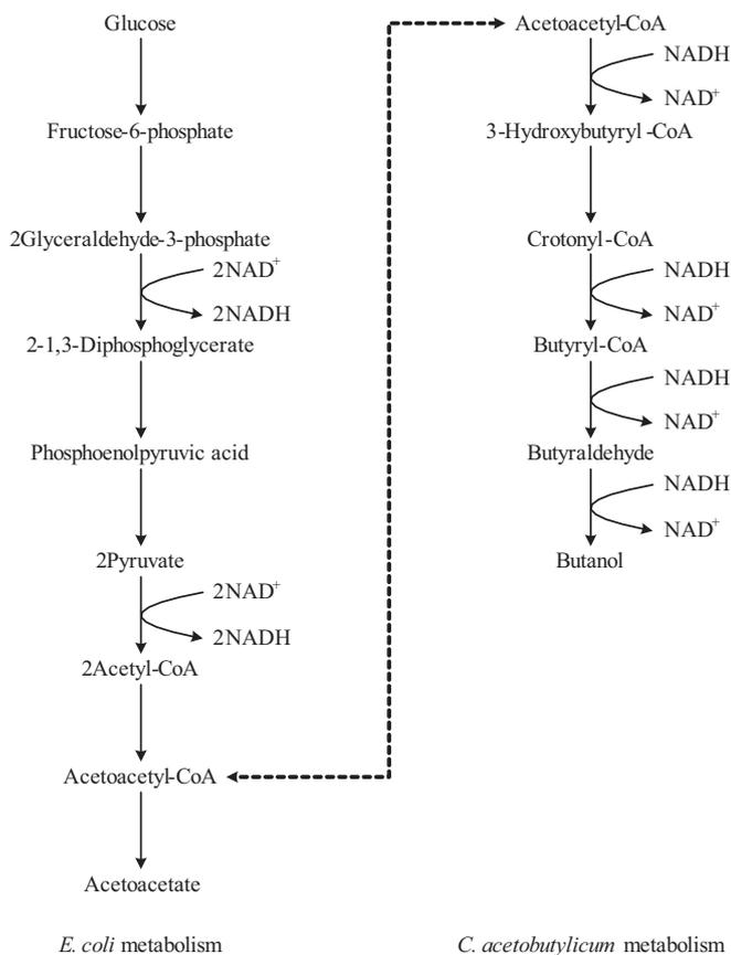
Fig. 3. Metabolic pathway map of butanol production through synthetic biology techniques. In both *E. coli* and *C. acetobutylicum* metabolisms, Acetoacetyl-CoA symbols connected by a bidirectional broken arrow represent the same metabolite.
