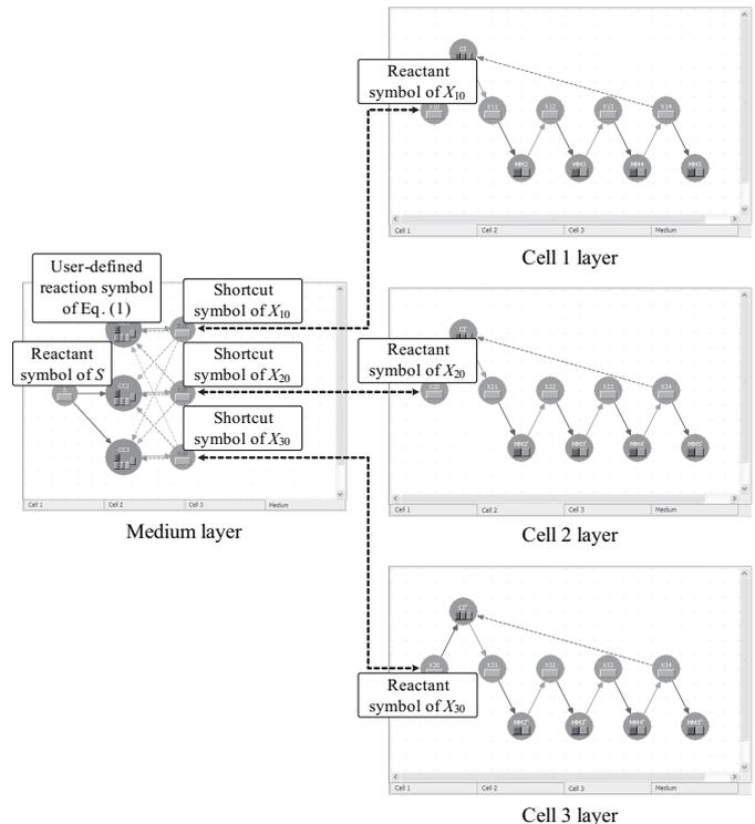
Fig. 7. Construction of reaction scheme for a simple model of cell–cell communication in WinBEST-KIT. A bidirectional broken arrow indicates the connection between a reactant symbol and its shortcut symbol.
