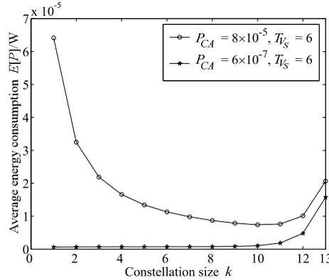
Figure 2: The average energy consumption  $E[P]$  vs. constellation size  $k$ .
