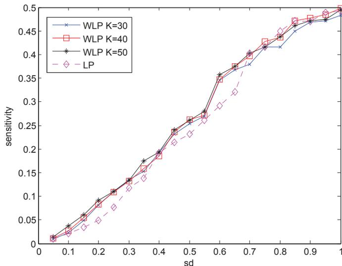
Fig. 2. Different settings of the parameter  $K$ . Performance of the WLP is not sensitive to different choices of  $K$ .
